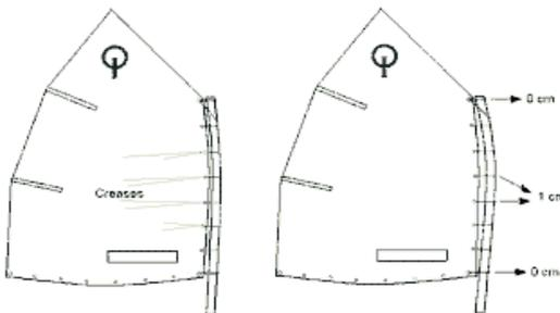
For luff tie adjustments maintain the luff between 1-2 mm distance between the sail & the mast.
