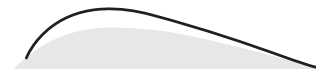
Shaded portion represents sail with tight headstay. Unshaded shows increased depth as headstay sags.
