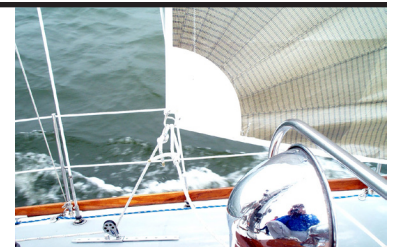
Set lead so that the sheet bisects the clew, applying approximately equal tension to leech and foot.
