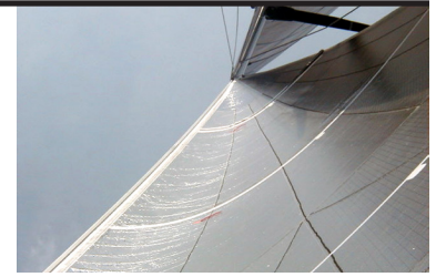
The appearance of horizontal wrinkles indicates correct halyard tension.
