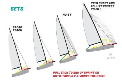
A SPINNAKER SOCK MAY BE USED TO KEEP THE SAIL FROM FILLING WHILE YOU HOIST. IF USING A SOCK, SECURE THE SOCK CONTROL LINES TO THE MAST AFTER HOISTING.
