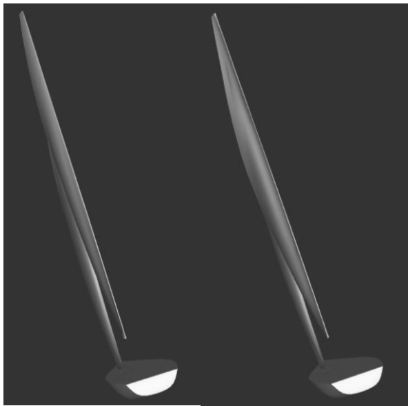
Figure 10 – Full Power and Depowered Trim: Simple Example
