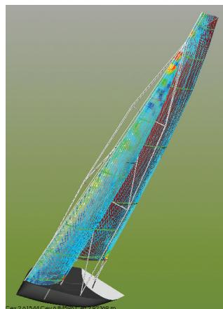
Stress, strain, loads and flying shapes are calculated in the Finite Element Modelling module
