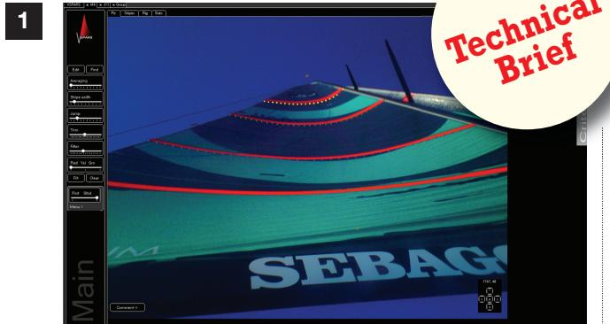
Before Racing, and when a new sail is hoisted, the first stop is the 'Main' page where the VSPARS program can be tweaked to ensure it's picking up correct draft stripes. The three dots (above the head, above the lower spreader, and above the 'B' in Seabag) frame the working area where the program looks for the draft stripes, which are bright orange or yellow. The yellow, blue, and green dots along the draft stripes are the data points the program uses to analyze the sail shape
