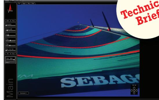
Before Racing, and when a new sail is hoisted, the first step is the 'Main' page where the VSPARS program can be tweaked to ensure it's picking up correct draft stripes. The three dots (above the head, above the lower spreader, and above the 'B' in Sebago) frame the working area where the program looks for the draft stripes, which are bright orange or yellow. The yellow, blue, and green dots along the draft stripes are the data points the program uses to analyze the sail shape
