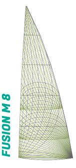
Fusion M 8 is designed specifically for super yachts. This totally customized product is tailored to the unique demands of the world's ultimate sailing machines. The ultra high-performance fiber-and-filament package features a customized blend of carbon and aramid or Vectran® and aramid to maximize performance and longevity. The Quantum super-yacht design team works hand-in-hand with each project from start to finish.
