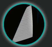
STEP 1 - SAIL SHAPE Define geometry of the sail and create mold shape using 3D design program and extensive database of boat and sail types.
