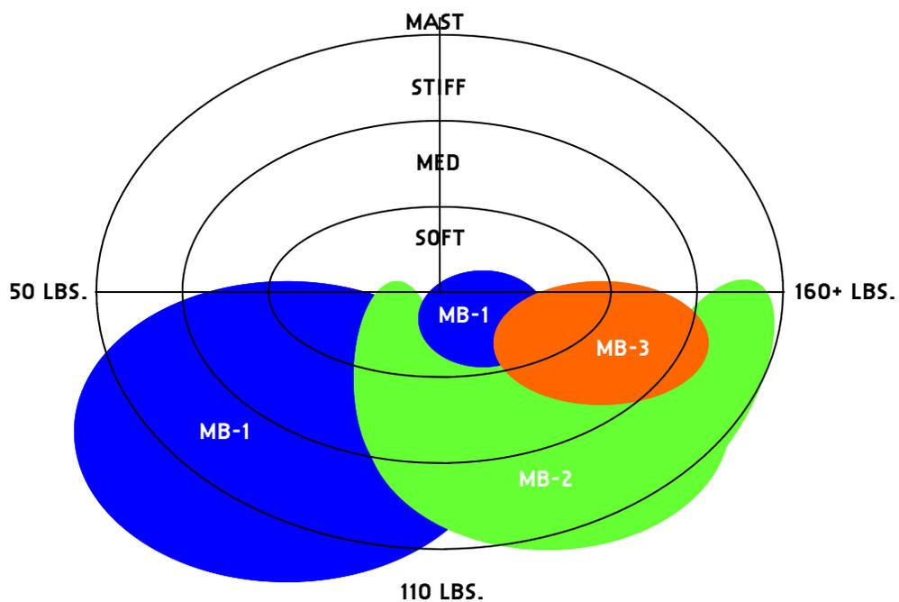
× Mast stiffness is how bendy your spar is in relation to a LeFeill Heavy Air, the benchmark to which all masts are compared.
